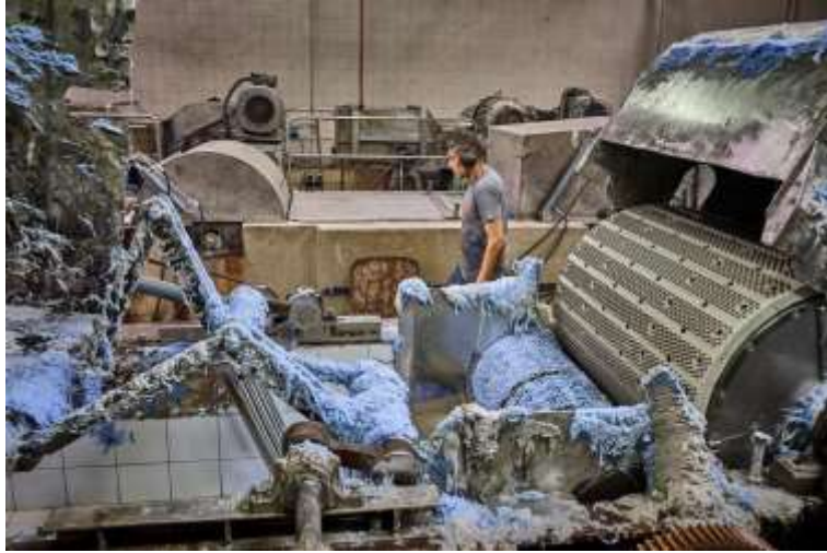
A worker next to a machine used for the “wet shredding” process, during which the old wool is washed and shredded
